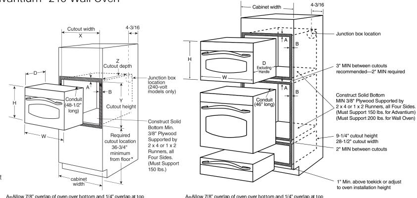
A=Allow 7/8" overlap of oven over bottom and 1/4" overlap at top edges of cutout. B=Allow 2-1/8" for overlap of oven over side edges of cutout.
