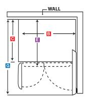
Allow 2" of clearance on hinge side of refrigerator when installing next to a wall where handle may make contact.
