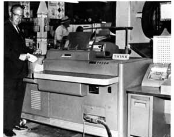
The IBM card is fed into this computer, which extends the quantities and prices, adds sales tax, totals and prints the sales ticket.
